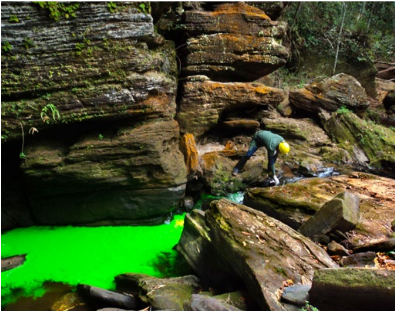
Injection of fluorescein tracer at the entrance of CAV-0001A, Morro do Pilar.
